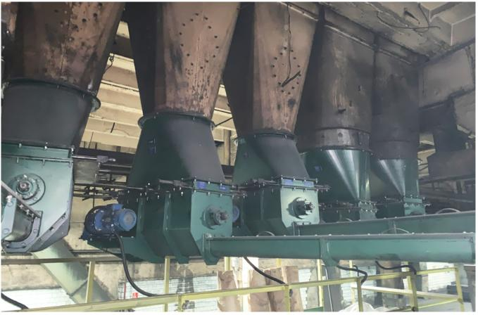
The soot supply line is a metal modular structure consisting of conveyors: scraper conveyor L=8,2m, scraper conveyor L=18m, scraper conveyor with two unloading L=18m, scraper conveyor L=22,5m, scraper conveyor L=24m, scraper conveyor L=25m, branch pipes and valves.
