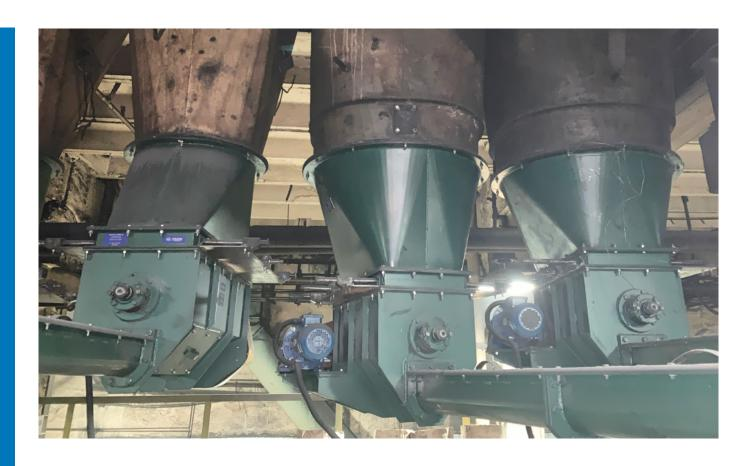
Conveyors in the line are connected to each other by branch pipes. Gates are installed on conveyors with two discharge nozzles. The loading section of the conveyors is equipped with a loading opening through which carbon black is received. On the tension section of each conveyor there is a mechanism with a sensor for monitoring the rotation of the scraper chain. The gate is equipped with 2 sensors to control the valve position.
